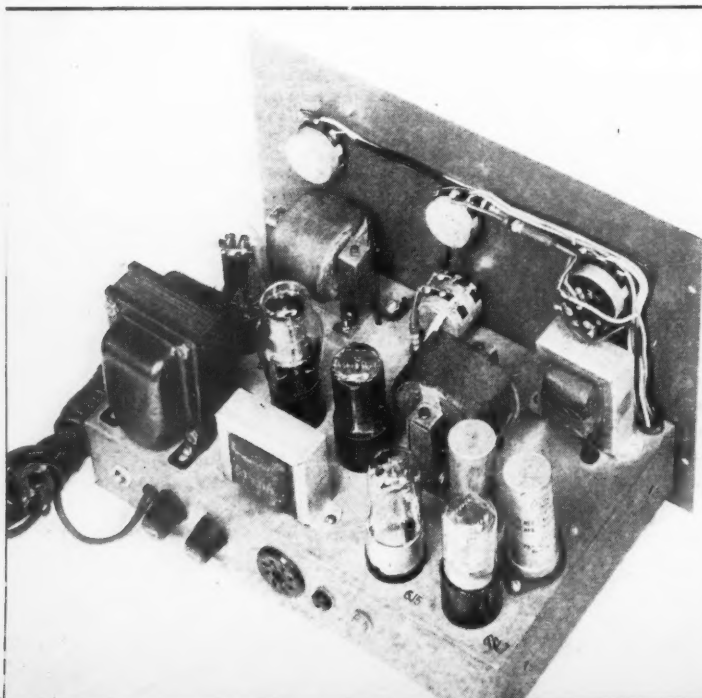
A view of the chassis layout. The two inductances in the audio filter circuit are the ones with the coils wound on the upper leg of the core. The socket for the detector-tube adapter extension is on the rear chassis wall.
